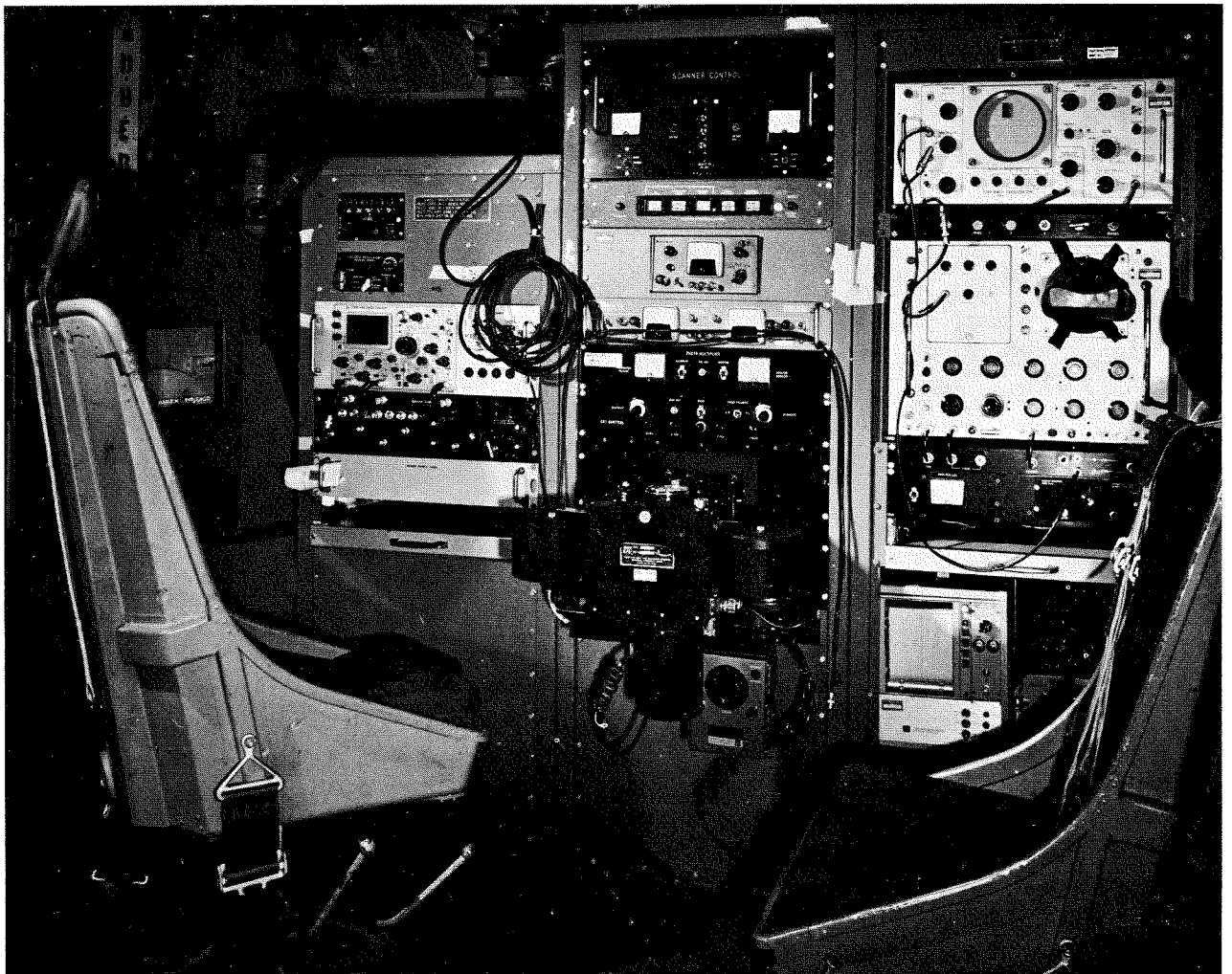
Fig. 1. MIAI thermal infrared scanner and recording unit as mounted in aircraft. Photograph by AFCRL.
