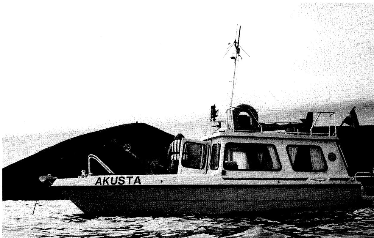
Fig. 1. The survey vessel in front of Surtla I. Surveys can be made at a speed of up to 12 knots; top speed in transit is 30 knots.
