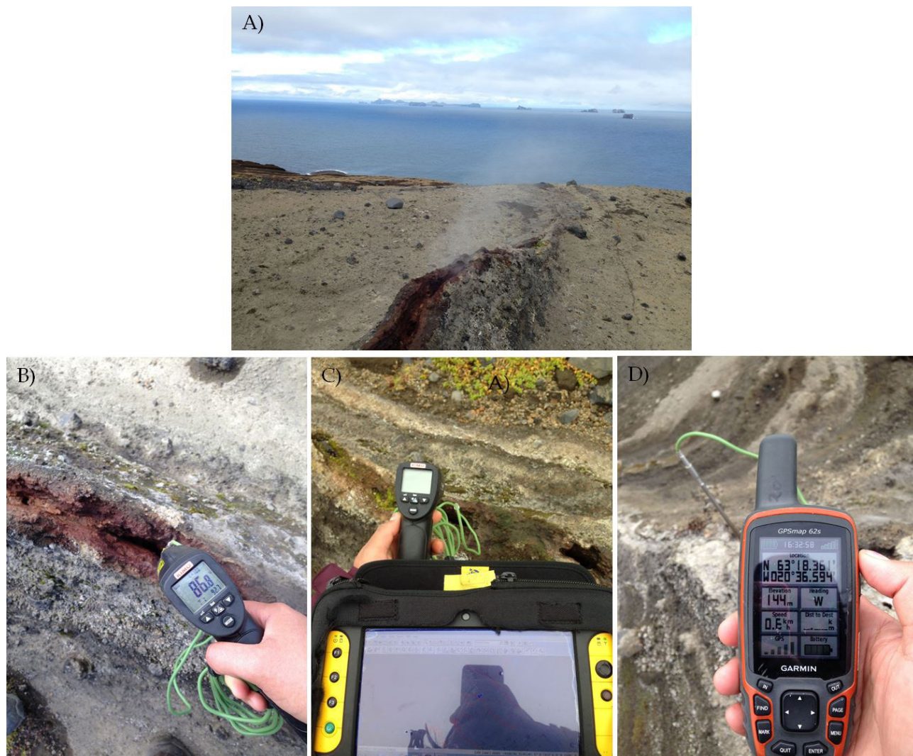
Figure 2. Images taken during the 2018 thermal survey: A) Photograph of a steaming fissure located at the top of Surtungur tephra cone (Vesturbunki). B) Temperature measurement taken with the thermocouple sensor-stick. C) Trimble tablet with integrated GPS allows logging of the temperature reading. D) Additional record of the temperature measurement coordinates made with handheld GPS.
