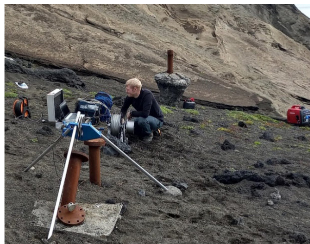
Figure 2. Photograph showing ÍSOR logging engineer conducting inclination measurements of the inclined borehole (SE-03) on August 5 th , 2021.
