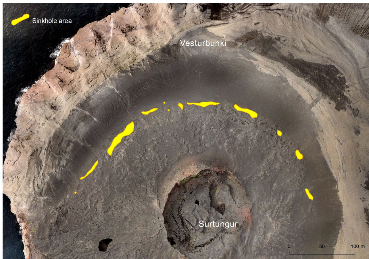
Figure 1. Distribution of sinkholes and tensional fissures along the lava margin within Vesturbunki. Orthoimage from 2023 (Natural Science Institute of Iceland, 2023. Unpublished data).
