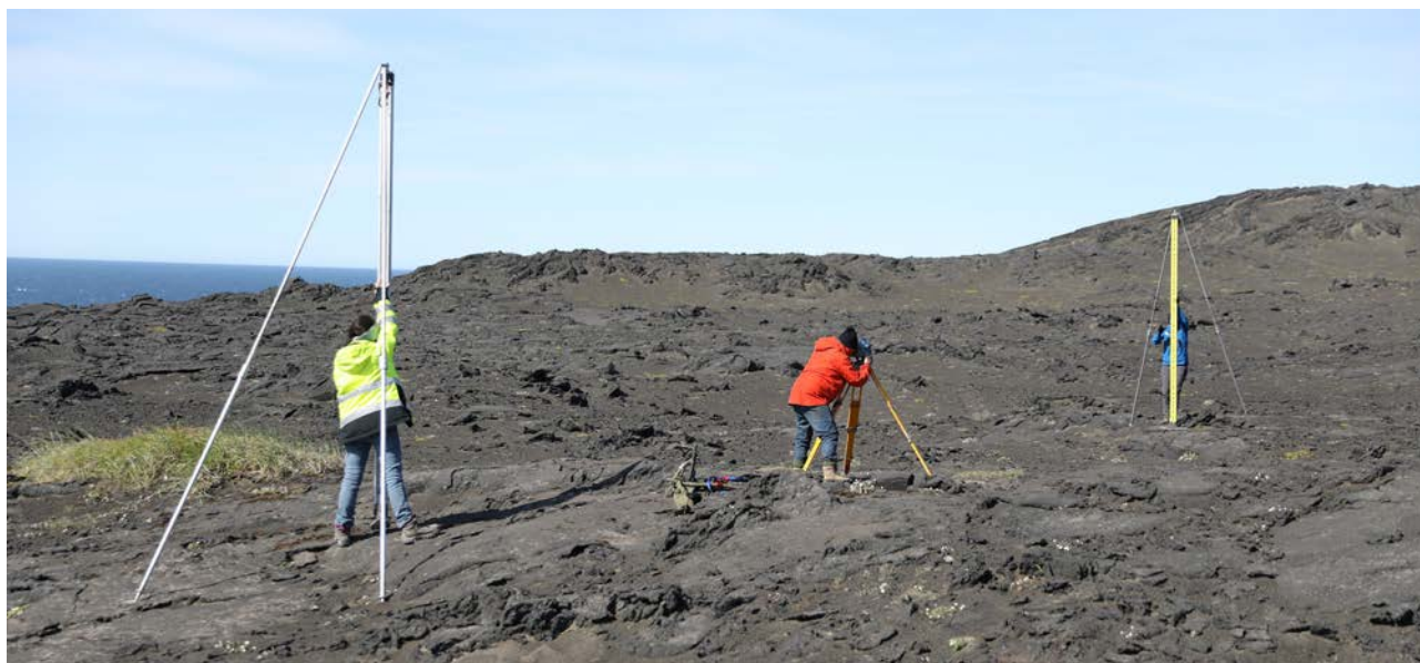
Figure 3. Levelling on Surtsey in 2023, the levelling instrument is located between the rods. The rod to the left is on a temporary benchmark to bridge between permanent benchmarks. The benchmark to the right is number 622. Photograph: Kristján Jónasson.
